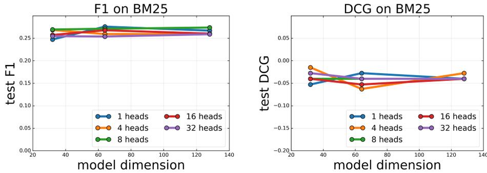
Figure 2: Performance on Robust04 BM25 for different model dimensions  $d$  and heads  $h$  ( $n_{\text{layers}} = 3$ ). We see strong and stable performance across different settings. Note that the y-axis is zoomed in to show details.
